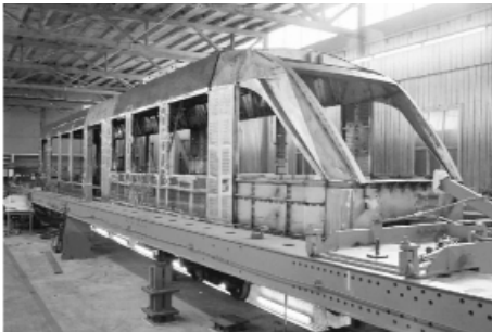
Illustration 1: Type testing car shell on pressure stand
